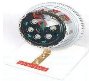
Fig: Cutaway Model Of Multi-Plate Clutch
