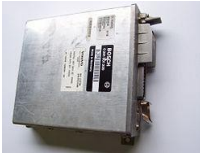
EDC control unit
